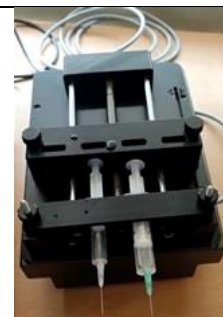
Figure 12: Multi Syringe Pump set up for purging fluids in micro-channels.
